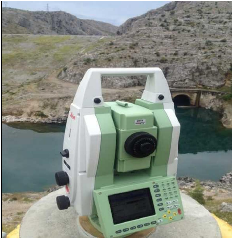
Figura 4-4 Instrument Station Total Leica tipi TM30 (M.Koço, 2015)
